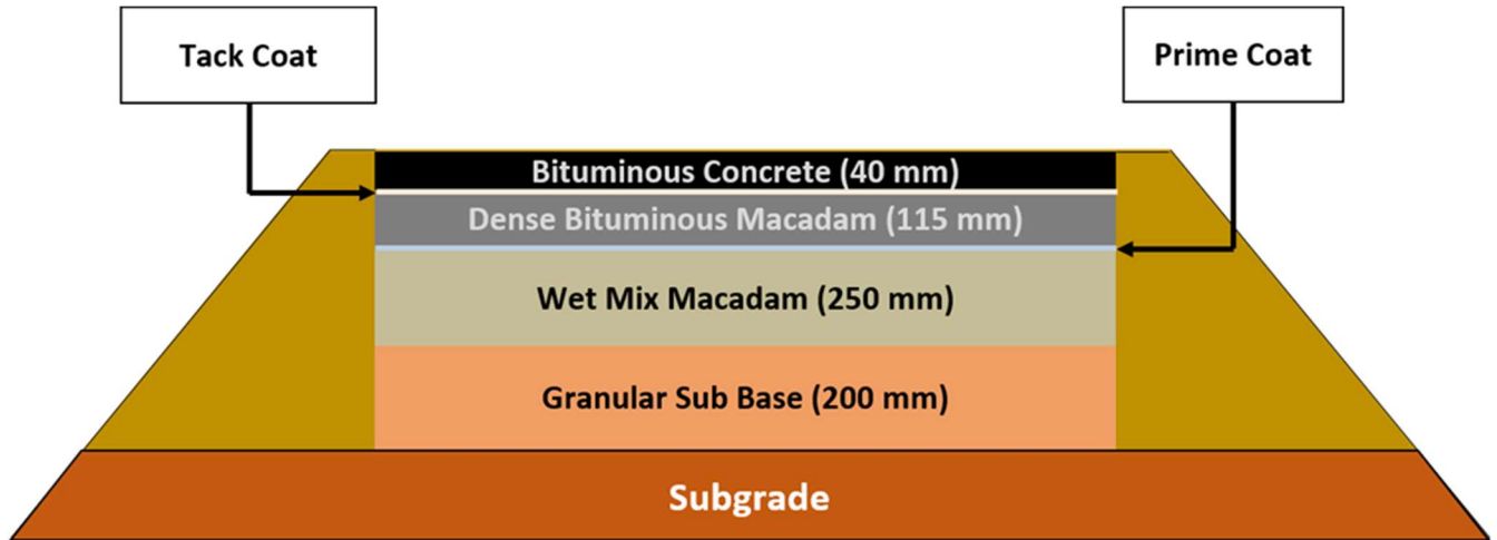
Conventional Design (IRC 37: 2018, Plate 4, CBR 8%, 50 MSA)
